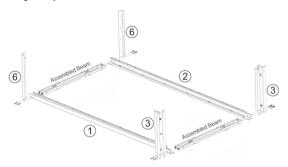
Using the remaining two Beams assembled in step 1, line up the other set of Left and Right Vertical Rails and fasten them to the Base and Top Brackets as shown.
